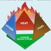
By removing any of these four things away, the fire will be extinguished.
